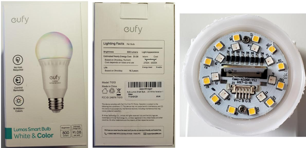
24. The Accused Infringing Devices contain a substrate, a cluster of LEDs, which are arranged two-dimensionally on the substrate and an interconnection circuit which is electrically connected to the LEDs.
