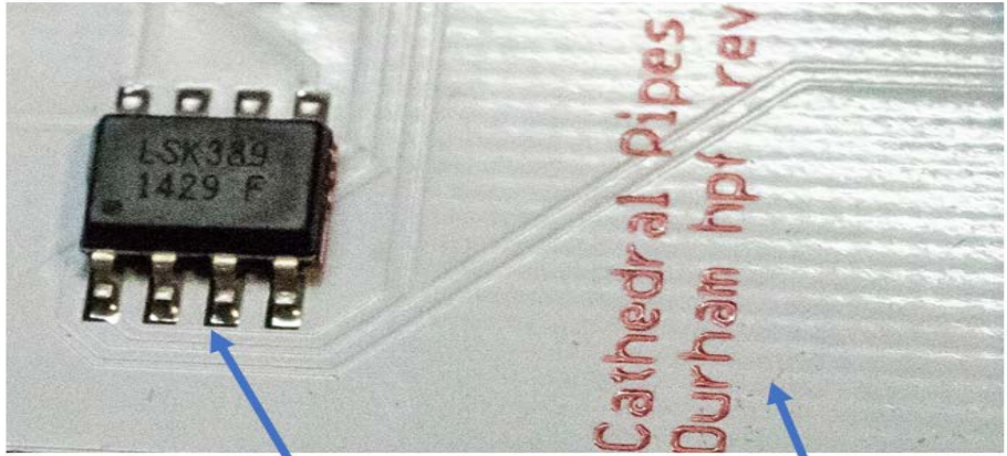
Evidence of one of two LSK389 chips on the Durham circuit board. Each LSK389 chip contains a pair of JFETs, which Cathedral Pipes connected in cascode per each JFET pair
