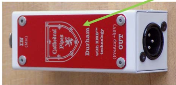
8 Durham's "...RC network including an additional resistor and an RF shunt capacitor; wherein the RC 9 network enables the phantom-powered JFET preamplifier gain circuit to be used as an external box powered 10 by the external phantom power supply to the microphone without radio frequency interference associated 11 with a cable length..."
