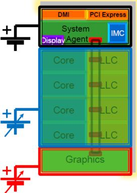
"wherein for at least some of the data processing units, the clock frequency is adjustable at runtime without affecting the clock frequency of at least one of: one other of the data processing units, and the bus system; and"
