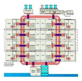
"wherein, in view of a probability of the chip having defects already when being manufactured, more of the plurality of data processing cores are implemented than used, so that some of the data processing cores can be exempted from data transfer via the bus system in response to a chip test."
