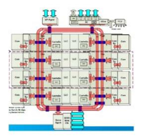
"each of at least some of the data processing cores includes a physically dedicated connection to at least one physically assigned one of the plurality of memory units, the assigned one of the plurality of memory units being accessible by another of the data processing cores via a secondary bus path of the bus system"
