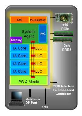
"the system further comprising: an interconnect system interconnecting each of the separated cache segments with each of the processors, each of the processors with neighboring processors, and each of the separated cache segments with neighboring separated cache segments"
