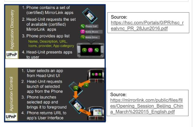
**Analyst comment-** Evidence demonstrates the advisor unit which mirrors the consumer electronic display on the vehicle dashboard. The evidence is taken from the MirrorLink official website, which shows the application control over the mobile phone to the vehicle infotainment system.
