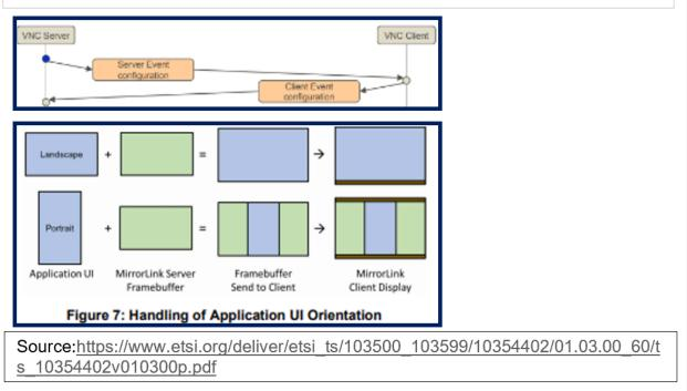
**Analyst comment-** Evidence demonstrates the handling of the user interface (display screen). The screen information is similar on the vehicle infotainment system and the MirrorLink associated smartphones.
