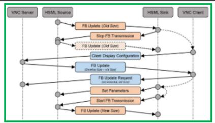
On reception of the ClientDisplayConfiguration message, the VNC Server shall send a FramebufferUpdate message containing a DesktopSize pseudo encoding rectangle with the new framebuffer resolution. In case the VNC Server does not support the new resolution, it shall send a FramebufferUpdate message containing a DesktopSize pseudo encoding rectangle with the old framebuffer resolution, as shown in Figure 14.
