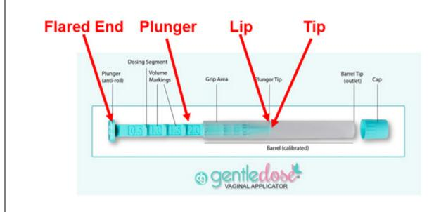
14 13. The plunger of the BiosRX's Gentle Dose® vaginal applicator is movable within 15 the hollow core between a dispensed position, a loaded position, and a filled position, wherein a 16 distance between the tip and the connector end in the loaded position is greater than a distance 17 between the tip and the connector end in the dispensed position and less than a distance between 18 the tip and the connector end in the filled position, as illustrated in part below:
