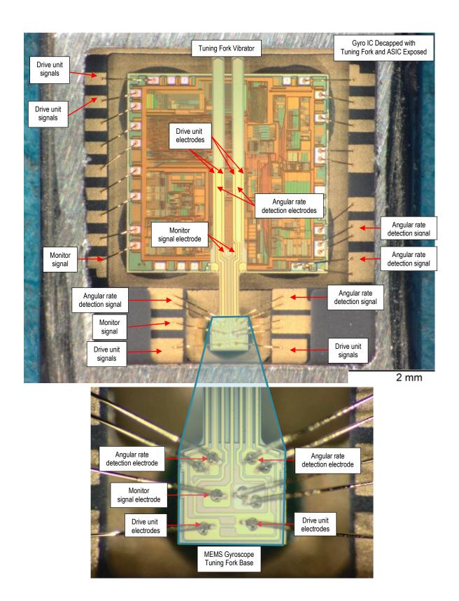
89. As one example, the Panasonic EWTS52AB gyroscope is shown below (note, the tuning fork tines broke off during decapsulation):
