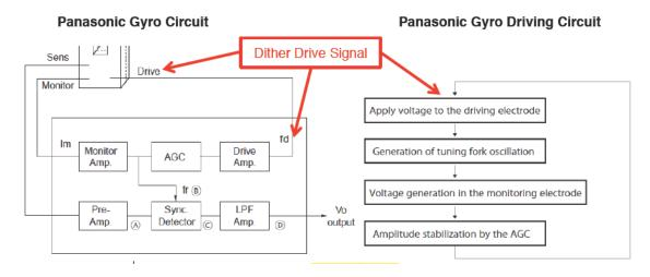
131. The Accused Gyroscopes utilize a Phase-Lock Loop ("PLL") in the digital processing system to control the phase and an Automatic Gain Control ("AGC") circuit to control the amplitude/magnitude.
