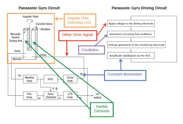
155. The movement (e.g., twisting) of the tuning fork tines due to rotation causes a capacitance change that is picked up by the sensing element's (e.g., Coriolis sensor) sensor that produces a voltage signal in response.
