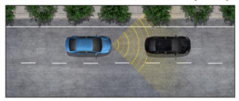
DRCC<sup>5</sup> is a high-tech cruise control system that uses a front grille-mounted radar and a forward-facing camera to detect vehicles in front of you and automatically adjust the vehicle's speed to help maintain a pre-set distance behind a vehicle ahead.
