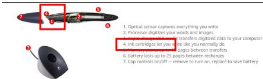
Figure 3. The Logitech IO2 has ink cartridges in the writing tip that allows users to write.
