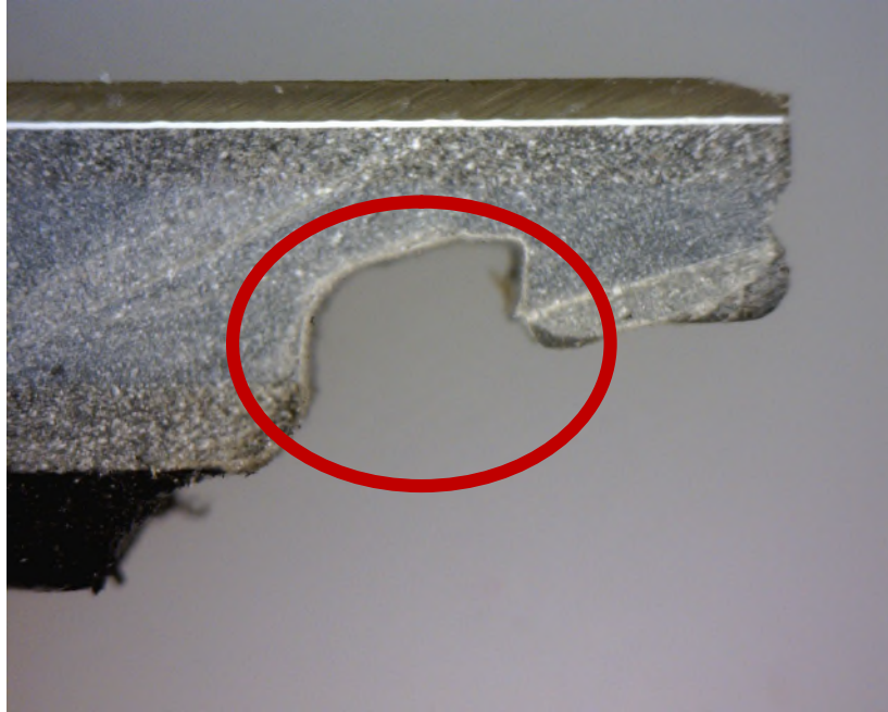
Downward Tongue Side of the Accused Locking Mechanism (downward groove circled)
