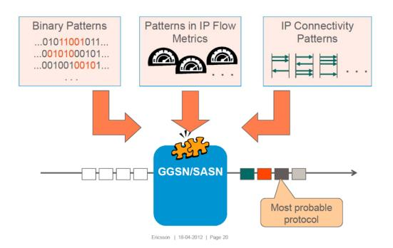
Integrated Policy Control & Charging Architecture for Mobile Broadband, at 20. Based upon the recognition of these patterns, the EPG is able to classify with a high degree of accuracy the application involved in the conversation flow:
