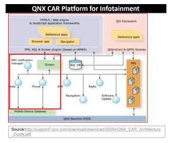
Analyst comment- Evidence demonstrates the architecture of the QNX CAR Platform for Infotainment, which shows the different stages for establishing communication from the mobile device to the vehicle infotainment system. The mobile phone is remotely connected using mobile device gateway.
