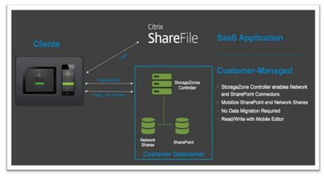
Figure 3. StorageZone Connector architecture
