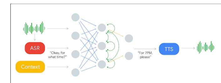
Incoming sound is processed through an ASR system. This produces text that is analyzed with context data and other inputs to produce a response text that is read aloud through the TTS system.
