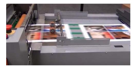
Ex. L (PDF of Duplo Ultra 300Ai High Speed UV Coater video presentation (*see* https://youtu.be/2LgAsSfcVbM?t=21) (showing a moving belt transporting paper within a Duplo Ultra 300Ai UV Coater at time 0:21 / 1:43)).
