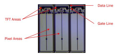
16. A TFT acts as a switch that operates its respective individual pixels using the circuity lines. In that way, the pixels can be turned on and off to create an image on an LCD by
