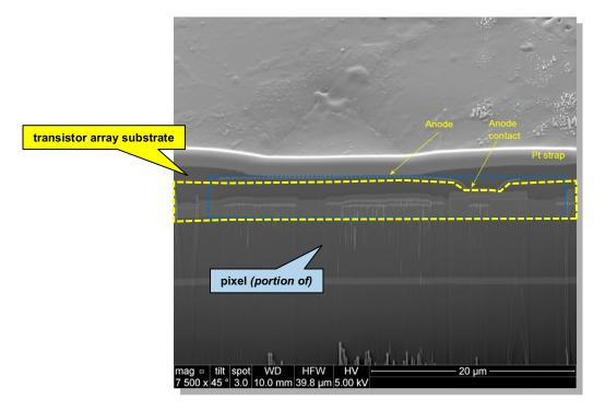
The transistor array substrate includes a plurality of pixels and comprises a plurality of transistors for each pixel, each of the transistors including a gate, a gate insulating film, a source, and a drain:
