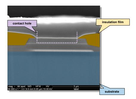
[1d] "at least one first electrode formed on said insulation film so as to cover said active elements, and connected to said active elements through said at least one contact hole, said at least one first electrode being made of a material which shields visible light;"
