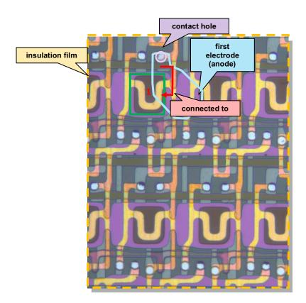
This electrode is formed of silver, which shields visible light.
