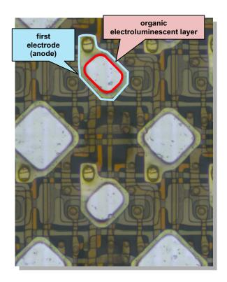
This organic electroluminescent layer emits in accordance with a voltage applied to the layer using the OLED cathode and anode.
