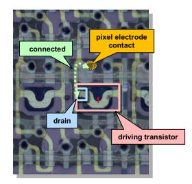
The plurality of transistors includes a switch transistor which makes a write current flow between the drain and the source of the driving transistor:
