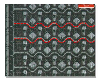
[1c] "a plurality of pixel electrodes for the plurality of pixels, respectively, the pixel electrodes being arrayed along the interconnections between the interconnections on the surface of the transistor array substrate;"
