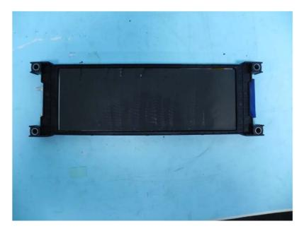
42. As shown below, the VISTA 2.0 Cell Module Assembly includes an adhesive pad disposed only within the frame of the partition member so that the frame completely surrounds the adhesive pad:
