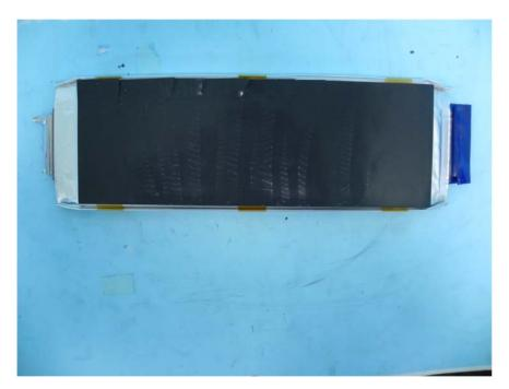
43. As shown below, in the VISTA 2.0 Cell Module Assembly, the adhesive pad is coextensive and in contact with the contact surface of the first and second unit cells.
