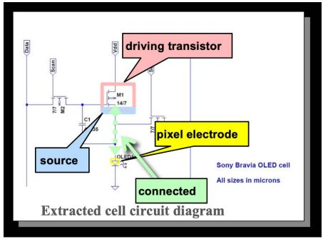
g. a plurality of light-emitting layers which are formed on said plurality of pixel electrodes, respectively. For example, the display panel of the Sony Bravia 55A1 OLED Television comprises a plurality of light-emitting layers that are formed on the pixel electrodes respectively, as shown below.
