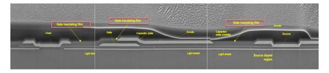
c. a plurality of signal lines which are patterned together with the gates of said plurality of driving transistors and arrayed to run in a predetermined direction on the substrate. For example, the display panel of the Sony Bravia 55A1 OLED Television comprises a plurality of signal lines that are patterned together with the gates of the driving transistors and arrayed to run in a predetermined direction on the substrate, as shown below.
