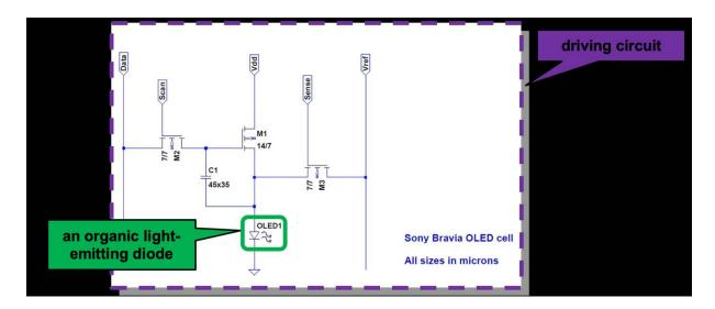
b. comprising a capacitor; a feedback coupling; a first thin film transistor as a current-driving transistor for the diode. For example, the driving circuits of the Sony Bravia 55A1 OLED Television have a capacitor, a feedback coupling, and a first thin film transistor as a current-driving transistor for the diode, as shown below.
