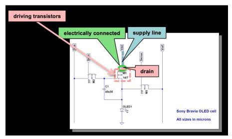
e. a plurality of feed interconnections which are connected to said plurality of supply lines along said plurality of supply lines. For example, the display panel of the Sony Bravia 55A1 OLED Television comprises a plurality of feed interconnections which are connected to the supply lines along the supply lines, as shown below.
