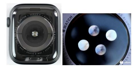
91. Claim 1 further recites: "a detection system located to receive at least a portion of the lens output beam reflected from the tissue." The Watches include a receiver, with multiple
