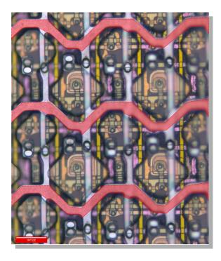
[1c] "a plurality of pixel electrodes for the plurality of pixels, respectively, the pixel electrodes being arrayed along the interconnections between the interconnections on the surface of the transistor array substrate;"
