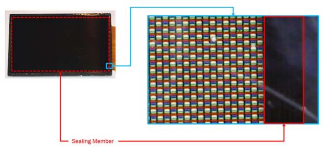
35. The Accused Panel shown below has a spacer in the seal to make a gap between the array substrate and the opposing substrate constant.
