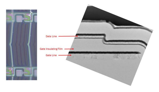
31. The Accused Panel also has a first interlayer film coating the data line and a first orientation film coating the first interlayer insulating film, as shown below.
