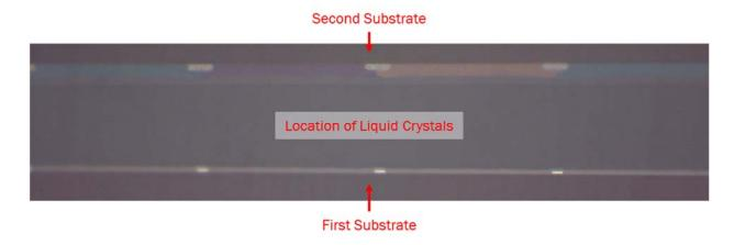
29. As shown below, the TFT-LCD Accused Panel contains a first substrate with a gate line, a common line parallel to the gate line.
