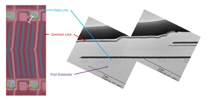
30. The Accused Panel has a data line intersecting the gate line with a gate insulating film between.
