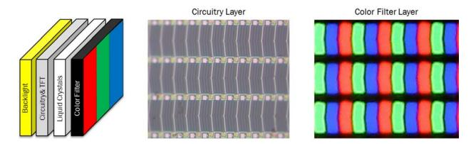
27. A thin-film transistor ("TFT") acts as a switch that operates its respective individual pixel using circuity lines. Using the TFT, each pixel can be turned on and off to create an image on a liquid panel display ("LCD") by allowing or preventing light to pass through. The individual pixels are more apparent when a color filter layer overlays the circuits as illustrated in the image below.
