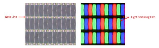
33. The Accused Panel shown below has a columnar spacer located above the gate line apart from the intersection of the gate and data lines.
