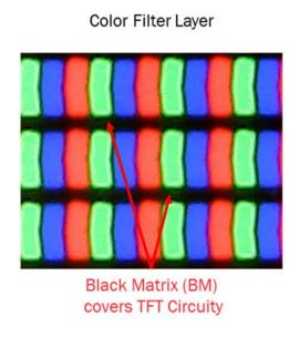
28. The Accused Panels have an active matrix type liquid crystal display device with two opposing insulating substrates and liquid crystal in-between, as illustrated below in reference to model no. LAM062M109A 2N6I519997 (utilized in the Nintendo Switch).
