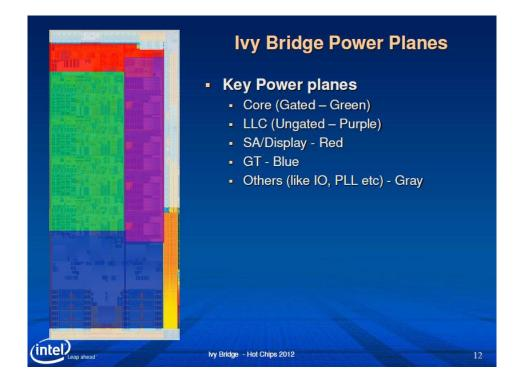
57. The on-chip power gates can only reduce the core (first) voltage from the supplied VCC power rail. When the core voltage (the first voltage) is above the operating voltage of the memory, the power gate will be fully opened, and the first voltage (core voltage) and the second voltage (VCC) will be the same. Thus, when the first voltage is above the minimum operating voltage of the memory, the first voltage will be provided to the memory array.
