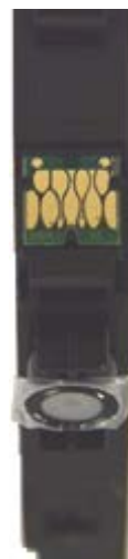
terminal arrangement viewed from vantage of printer's contact forming members . . . with the exit of the ink supply opening facing downwards
