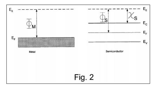
43. Schottky was wrong. In reality, the Schottky barrier at a metal-semiconductor junction is generally different than Schottky's equation would predict. The energy-band diagram below from the patents illustrates an increased Schottky barrier at a metal-semiconductor junction.
