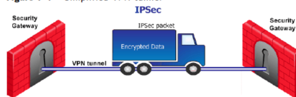
Figure 7-1 Simplified VPN tunnel
