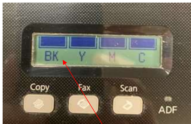
memory device shows, on the printer's display screen, the amount of black ink remaining in the Representative '749 Ink Cartridge
