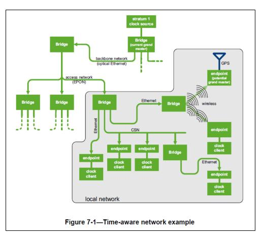
(Source: IEEE Standard for Local and metropolitan area networks - Timing and Synchronization for Time - Sensitive Applications in Bridged Local Area Networks - IEEE Std 802.1AS<sup>TM</sup>-2011)
