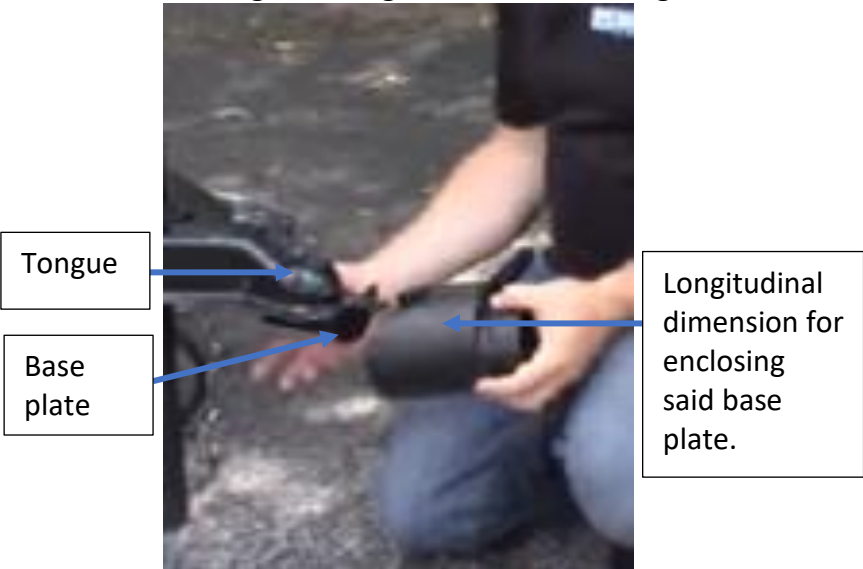
Figure 24B: Box Housing Enclosing Base Plate and Tongue
