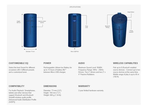
27. BOOM 3 (i.e., information appliance) is configured to transmit control signals (e.g., play, pause, skip track) to the mobile device (i.e., personal computer) via Bluetooth (i.e., the bi-directional communication link). The control signals (e.g., play, pause, skip track)
