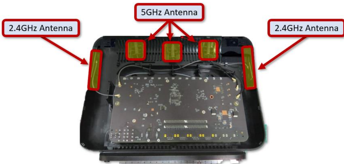
Nokia 7368 ISAM ONT G-240W-B Antennas, DEVICE TEARDOWN IMAGE (annotation added) (showing the antennas in the device).
