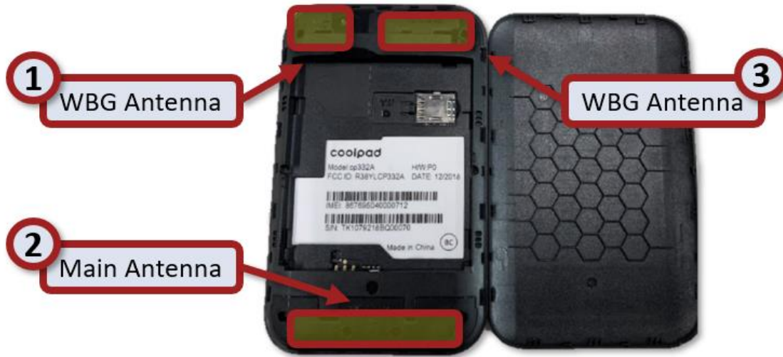
Sprint Coolpad Surf 2.4GHz Antennas, DEVICE TEARDOWN IMAGE (annotation added) (showing the three antennas in the device).
