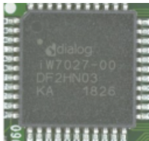
[Dialog iW7027 on LED Control Board in Hisense 55H9F]
