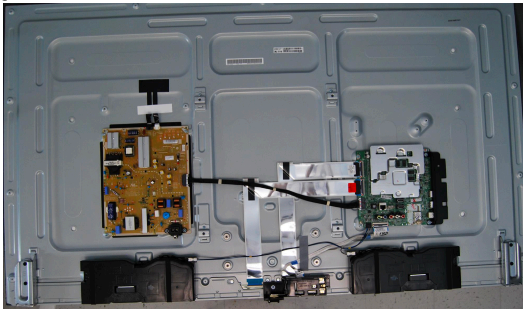
28 [LED Control Board/Power Board and Mainboard for LG 55UJ7700]
