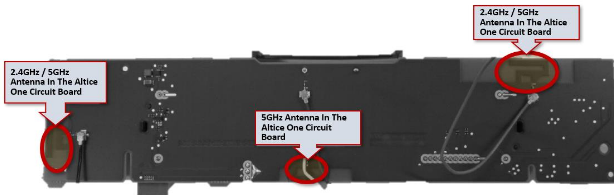
Altice One WiFi Antennas, ALTICE ONE TEARDOWN IMAGE (annotations added).
