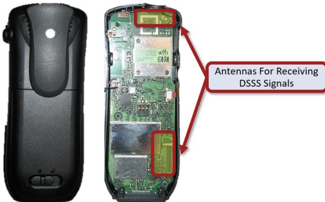
Mitel 5624 2.4GHz Antenna Location, DEVICE TEARDOWN IMAGE (annotation added).
