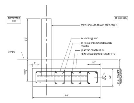
55. Upon information and belief, the Thornton Tomasetti/Weidlinger bollards have "a plurality of structural members," which include reinforced concrete footing, steel channel members, and steel plates, or the equivalent thereof. Upon further information and belief, these structural members intersect with each other and are tied together, or the equivalent thereof, as seen below:
