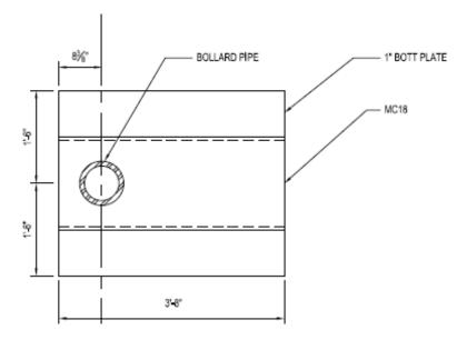
57. Upon information and belief, the Thornton Tomasetti/Weidlinger shallow mount bollards are secured to the channel members and the plate, shown below, and extends upwardly from the base so as to transmit forces applied to the at least one bollard to the base, or the equivalent thereof.
