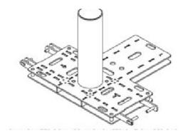
174. Upon information and belief, Ameristar's shallow mount bollards have "a plurality of structural members which intersect and are tied together." As can be seen in the drawings below, there are numerous structural members, including but not limited to the base plates, link arms, and rebar, which intersect and are connected to one another, or the equivalent thereof:
