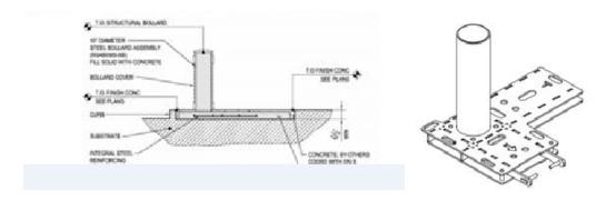
177. Upon information and belief, the base of Ameristar's shallow mount bollards have been configured to be mounted in a shallow excavation with at least one bollard extending above grade, or the equivalent thereof. The name of its product is "Ultra Shallow Mount Bollards," and
