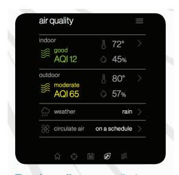
The **air quality screen** displays indoor air quality levels (when a Daikin *One* home air monitor is connected), outdoor air quality, and weather (when connected to the internet).
