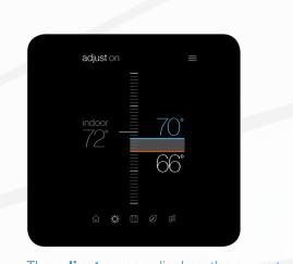
The **adjust screen** displays the current temperature on the left and set-points on the right. Change the set-points by dragging them or by turning the dial.
