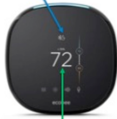
Temperature measurement from structure conditioned by HVAC system (i.e., room temperature)
