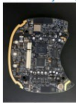
HVAC control system (Ecobee4 circuit board assembly)
