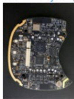
HVAC control system (Ecobee4 circuit board assembly)
