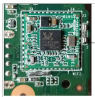
Wireless communication chip positioned on said substrate
