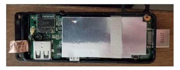
The Accused Productsality includes a wireless communication chip (e.g. AW-NB168sm board including Realtek RTL8723BS Combo Module) which is a wireless communication chip capable of communication over Bluetooth and Wi-Fi.
