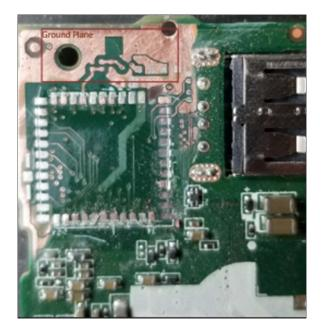
a wireless communication chip electrically connected to said ground plane and proximate thereto;
