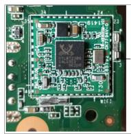
Wireless communication chip positioned on said substrate
