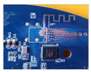
The Accused Instrument utilizes an antenna that is electrically coupled to the wireless communication chip and electrically shorted at one end to said ground plane:
