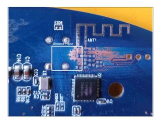
Both the Ground Plane and RF Chip are position on the substrate
