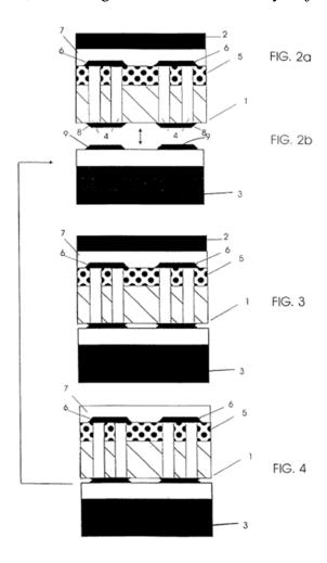
15. In the above embodiments, Figures 2a and 2b show a first and second substrate as recited in Claim 1. Figure 3 illustrates the via holes and the connections between the first and second substrates. Figures 3 and 4 also illustrate the contact areas and lands (8 and 9) identified and included in Claim 1. The first and second semiconductor substrates are connected in such a
