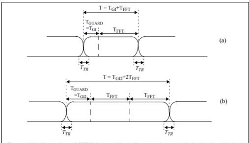
Figure 108—Illustration of OFDM frame with cyclic extension and windowing for (a) single reception or (b) two receptions of the FFT period
