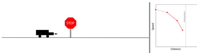
Figure 1: (Left) Expected behavior of a driver when encountering a stop sign. (Right) Expected velocity over distance of the driver when encountering a stop sign.
