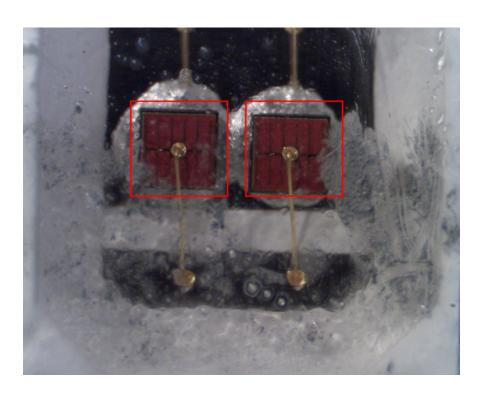
As another example, a cross-sectional view of a phosphor LED chip from a Kasa Smart Wi-Fi LED Bulb is shown with respect to claim element 1(c) below.
