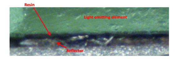
1(f): wherein a face of the reflector on that reflects a light beam outgoing from the light emitting element is formed into a rough surface.— In the Kasa Smart Wi-Fi LED Bulb, a face of the reflector that reflects a light beam outgoing from the light emitting element is formed into a rough surface.
