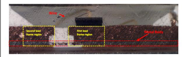
As another example, this configuration is shown in the below image of a cross-sectional view of a phosphor LED chip from a Kasa Smart Wi-Fi LED Bulb:
