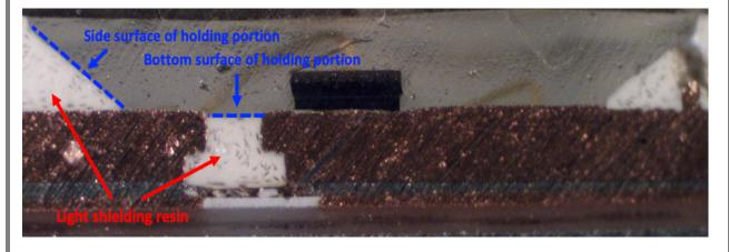
As another example, shown below is the cross-sectional view of the phosphor LED chip from the Kasa Smart Wi-Fi LED Bulb with the light shielding resin covering a bottom surface and a side surface of the holding portion identified:
