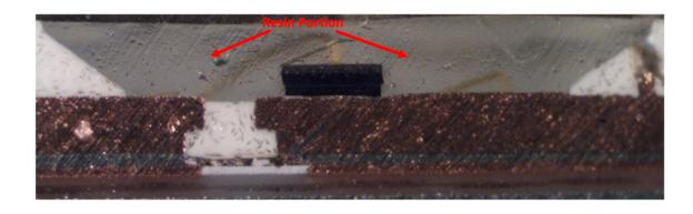
As another example, shown below is a cross-sectional view of a phosphor LED chip from a Kasa Smart Wi-Fi LED Bulb with a resin portion surrounding the circumference of the LED chip and fastening first and second lead frames identified:
