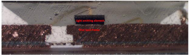
As another example, shown below is the cross-sectional view of the phosphor LED chip from the Kasa Smart Wi-Fi LED Bulb with an identification of a first lead frame on which the semiconductor light emitting element is mounted:
