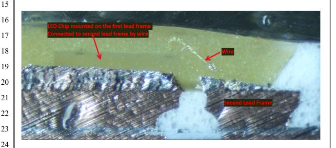
1(e): a resin portion surrounding a circumference of said LED chip, and fastening said first and second lead frames,— The Kasa Smart Wi-Fi LED Bulb comprises a resin portion surrounding the circumference of the LED chip and fastening the first and second lead frames.
