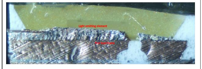
1(d): a second lead frame electrically connected to said semiconductor light emitting element via a wire, and — The Kasa Smart Wi-Fi LED Bulb comprises a second lead frame electrically connected to the semiconductor light emitting element via a wire.
