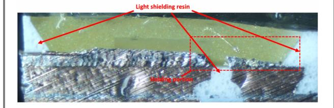
1(g): wherein said light shielding resin has a reflectance higher than a reflectance of said light transmitting resin, and —In the Kasa Smart Wi-Fi LED Bulb, the light shielding resin has a reflectance higher than a reflectance of the light transmitting resin.
