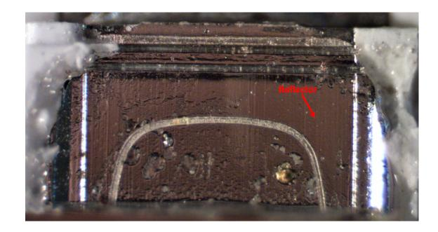
1(e): a resin disposed between the light emitting element and the reflector on the substrate,— The Kasa Smart Wi-Fi LED Bulb comprises a resin disposed between the light emitting element and the reflector on the substrate.
