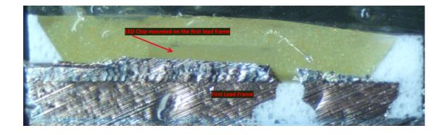
1(d): a second lead frame electrically connected to said LED chip via a wire, and — The Kasa Smart Wi-Fi LED Bulb comprises a second lead frame that is electrically connected to the LED chip via a wire.
