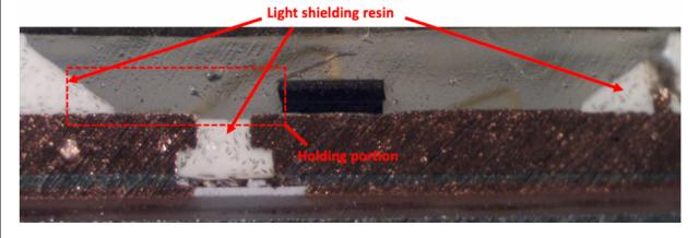
As another example, shown below is the cross-sectional view of the phosphor LED chip from the Kasa Smart Wi-Fi LED Bulb with the light shielding resin and holding portion identified:
