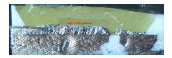
1(c): a first lead frame on which said semiconductor light emitting element is mounted, — The Kasa Smart Wi-Fi LED Bulb comprises a first lead frame on which the semiconductor light emitting element is mounted.
