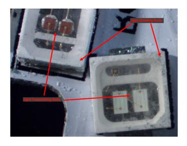
1(h): wherein said light shielding resin is formed to cover a bottom surface and a side surface of said holding portion provided in said light transmitting
