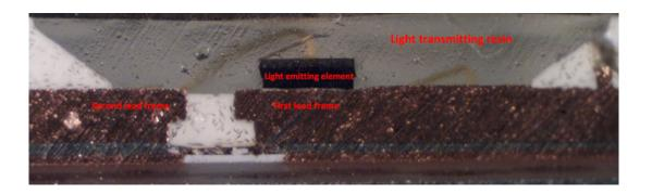
As another example, shown below is the cross-sectional view of the phosphor LED chip from the Kasa Smart Wi-Fi LED Bulb with the light transmitting resin formed on the light emitting element and first and second lead frames identified:
