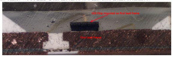
As another example, a cross section of a phosphor LED chip from a Kasa Smart Wi-Fi LED Bulb was taken, and a resulting cross-sectional view is shown below with the phosphor LED chip mounted to a first lead frame identified:
