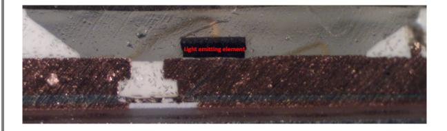
As another example, a cross section of a phosphor LED chip from a Kasa Smart Wi-Fi LED Bulb was taken, and a resulting cross-sectional view is shown below with a semiconductor light emitting element identified:
