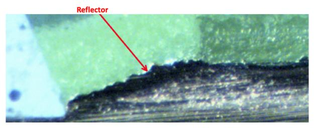
To further illustrate the presence of the reflector on the substrate in the Kasa Smart Wi-Fi LED Bulb, below is a top-down view of a phosphor LED from a Kasa Smart Wi-Fi LED Bulb with the phosphor layer removed and the reflector identified:
