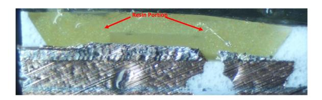
1(f): wherein a metal body is located under a region of said first lead frame where said LED chip is mounted, and wherein the second lead frame has a portion where the wire is connected and the metal body is provided to extend to a region below said portion of the second lead frame.— In the Kasa Smart Wi-Fi LED Bulb, a metal body is located under a region of the first lead frame where the LED chip is mounted and the second lead frame has a portion where the wire is
