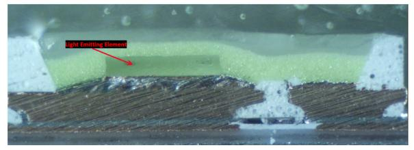
1(d): a reflector on the substrate for reflecting a light beam outgoing from the light emitting element; and— The Kasa Smart Wi-Fi LED Bulb comprises a reflector on the substrate for reflecting a light beam outgoing from the light emitting element.
