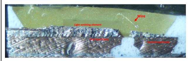
1(e): light transmitting resin formed on said semiconductor light emitting element and on said first and second lead frames, — The Kasa Smart Wi-Fi LED Bulb comprises a light transmitting resin formed on the semiconductor light emitting element and on the first and second lead frames.
