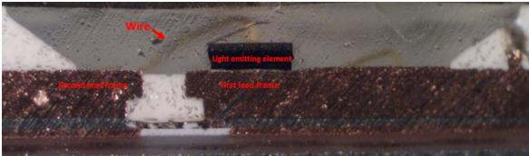
As another example, shown below is the cross-sectional view of the phosphor LED chip from the Kasa Smart Wi-Fi LED Bulb with the second lead frame electrically connected to the semiconductor light emitting element via a wire identified:
