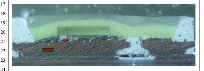
1(c): a light emitting element on the substrate;— The Kasa Smart Wi-Fi LED Bulb comprises a light emitting element on the substrate.
