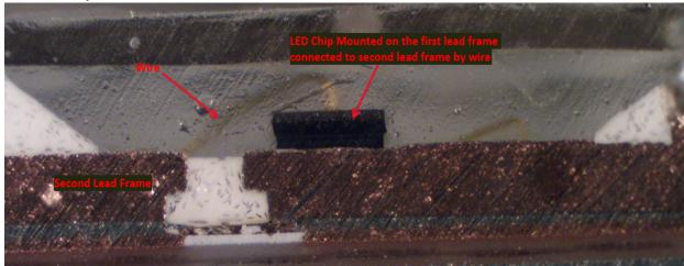
As another example, shown below is a cross-sectional view of a phosphor LED chip from a Kasa Smart Wi-Fi LED Bulb with a second lead frame electrically connected to a first lead frame via a wire identified:
