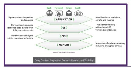
Traditional sandboxes have visibility down to the operating system level only. Forcepoint offers a unique isolation and inspection environment that simulates an entire host including the CPU, system memory and all devices. Deep Content Inspection interacts with malware to observe all the actions it might take within this complete environment, and even identifies 'dormant code' for special analysis."
