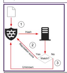
When a file transfer matches a rule in the File Filtering Policy that applies the Cloud Sandbox scan, the NGFW Engine sends a hash of the file to the Cloud Sandbox.
