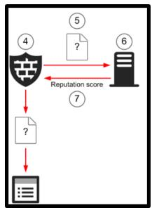
5 If the file has not previously been analyzed, the NGFW Engine uploads a copy of the unknown file to the sandbox server. If any of the files in a .zip archive have not previously been analyzed, the NGFW Engine uploads a copy of the whole .zip archive to the sandbox server.
