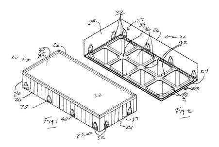
37. Figures 1 and 2 of the '150 Patent show a bed having a molded outer shell with a top, bottom, two sides with support ridges, two ends with support ridges, mounting flanges in the side and end walls and adjacent the bottom, and recessed pockets in the top and bottom. The mounting flanges comprise bolt holes extending through the bottom.
