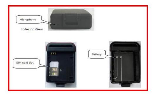
User can access the interior part of body for replacing battery and putting SIM card.
