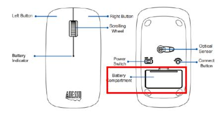
As shown above, the IMOUSE M300W includes a body including an opening for accessing interior of the body to place batteries within the housing.
