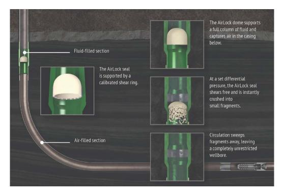
10. The AirLock® system (above in green) is a tubular body attached to the casing string (above in grey). Within the tubular is a rupture disc (above in white). The portion of the casing string above the rupture disc is filled with fluid. The portion of the casing string below the rupture disc is filled with air, which creates buoyancy in the lower portion of the string. This
