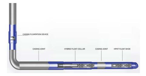
13. According to Innovex's marketing materials, the Casing Floatation Device allows casing to be floated in the casing string, significantly reducing friction which allows the casing to
