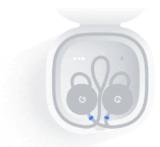
66. The magnetized pockets formed in the Pixel Bud case are configured to hold the earbuds firmly in place.
