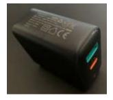
48. The products also include a power converter that converts the voltage from the electrical outlet to a voltage that can be output from the charging adapter. For example, some of the Accused Products can be connected to an AC electrical outlet and convert the AC voltage to a DC voltage. Other Accused Products can be connected to an electrical outlet in a vehicle and convert power from 12v to 5v for output from the charging adapter.
